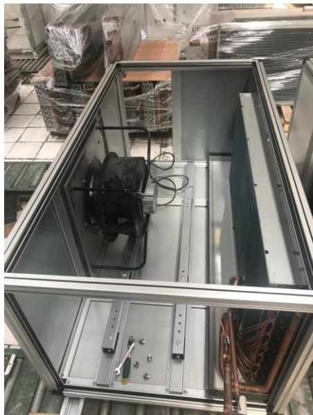
Figure 1: Location of EC Motor on the old box
